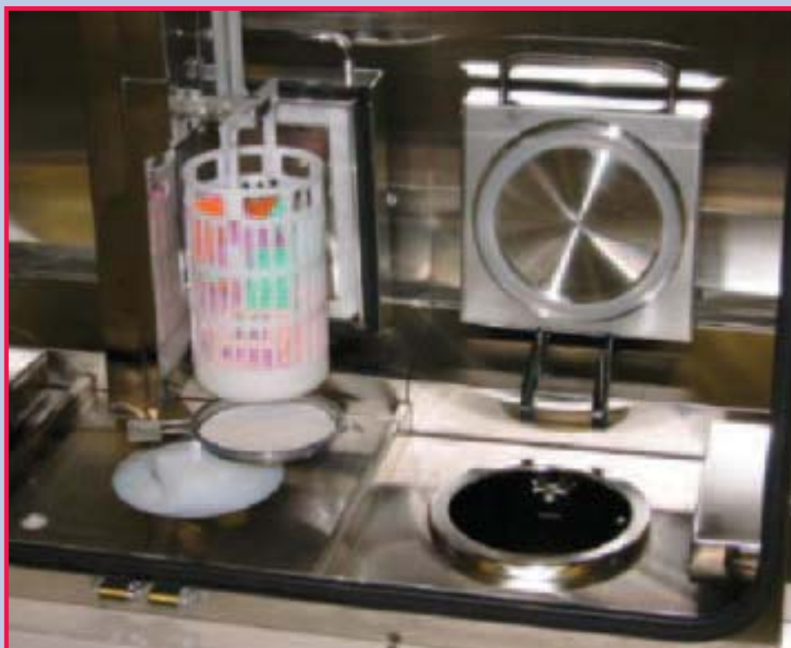
Fig. 3. Shown in this photograph is the transfer of samples from a microwave chamber to a vacuum retort of the Continuous Rapid Tissue Processor. The cassettes with their respective tissue samples are shown in the basket, which is transported from one station to the next by a robotic arm.
